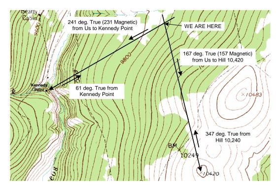
Figure 11: Bearings and Triangulation
